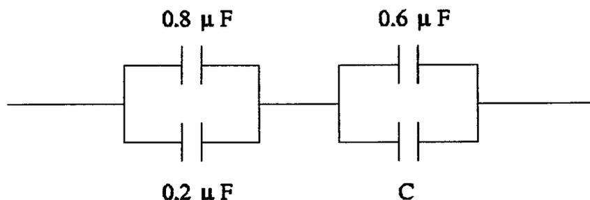
(c) Consider the system of two capacitors shown in the picture. Determine the magnitude of the voltage across each capacitor.
