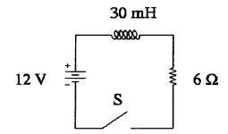
i. Find the time constant  $\tau$  of the system[2]ii. Calculate the current in the circuit at t = 2 ms[3]iii. Find the voltage across the resistor after one time constant  $t = \tau$ [3]PHYS1B26/2005PLEASE TURN OVER
