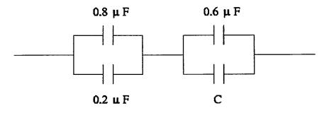
(c) Consider the system of two capacitors shown in the picture. Determine the magnitude of the voltage across each capacitor.
